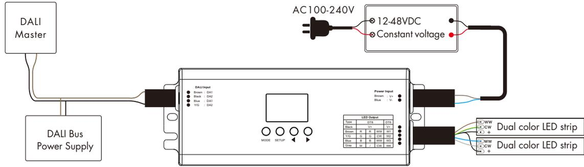
Note: The 3/4 LED channel output is same as 1/2 LED channel.
