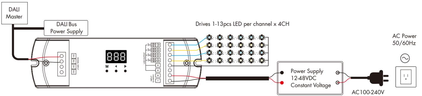
Note: The 3/4 LED channel output is same as 1/2 LED channel.
